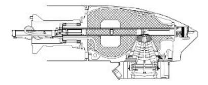
The design of the GammaBeam 100-80 head meets the international standards for source shielding, radiation transmission and radiation leakage. The dual control system monitors the source position and automatically retracts the source if a problem with source travel or position is detected. Operators and patients can feel conf dent that the GammaBeam 100-80 has been designed with their safety in mind.
