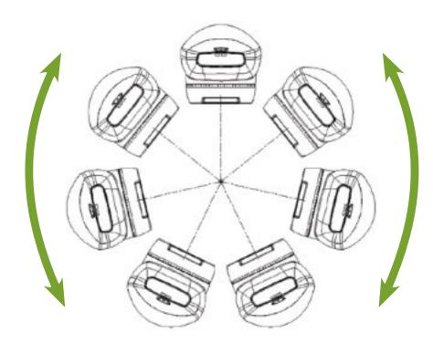
The Theratron® Equinox™ control system automatically calculates the arc speed based on the arc angle and treatment time. This makes the delivery of any arc treatment a simple matter of entering the time and angle. In addition, this feature makes it possible to perform serial tomotherapy using the nomosSTAT™ from Best® NOMOS®.
