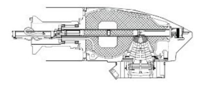
The design of the Theratron® Equinox™ head meets the international standards for source shielding, radiation transmission and radiation leakage. The dual computer control system monitors the source position and automatically retracts the source if a problem with source travel or position is detected. Operators and patients can feel confident that the Theratron® Equinox™ has been designed with their safety in mind.
